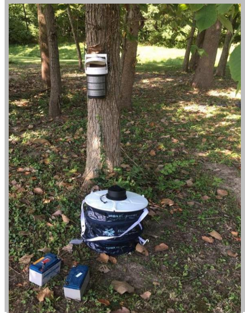
Fig. 1: image of the BG Sentinel trap (on the ground) to collect adult female mosquitoes and an oviposition container (on the tree) used to collect eggs.
