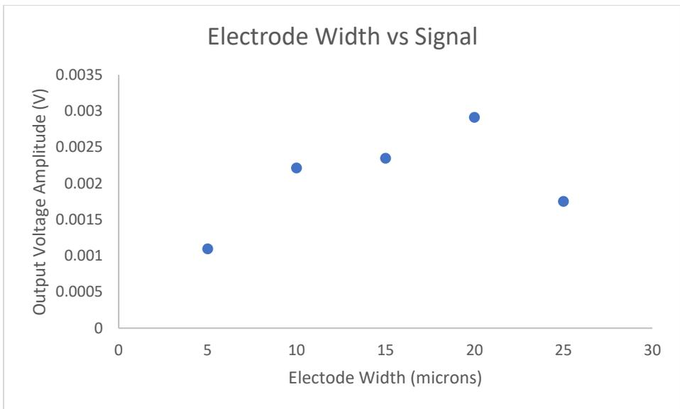
Fig. 15 Electrode width vs output voltage amplitude for second of the bipolar peaks
