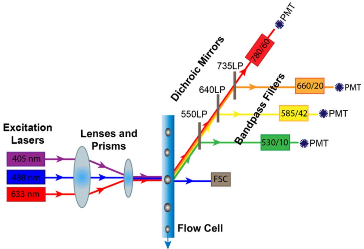
Fig. 1 Schematic showing mechanism of a flow cytometer. Cells are conjugated with fluorophores and focused into a single file line. Lasers are selected based on the fluorophore tag and used to excite the fluorophores on the cells. The intensity of light emitted by the fluorophores on a given cell can be correlated with the amount of the protein of interest on the surface of that cell. [15]
