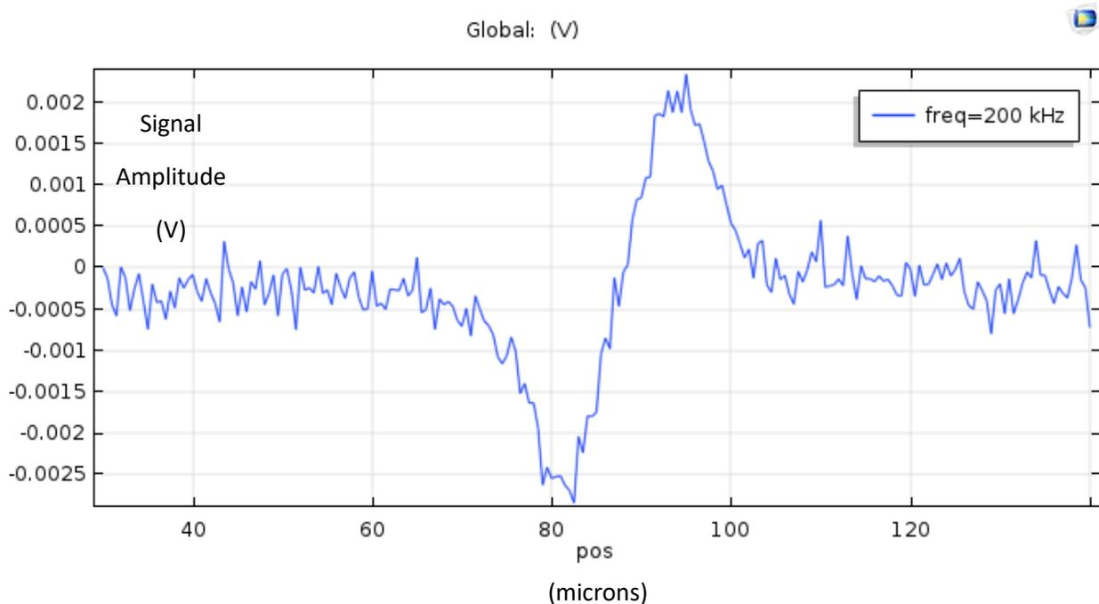
Fig. 9 Graph of voltage difference against x position for control test. Shows bipolar pulse similar to what can be seen in Fig. 3
