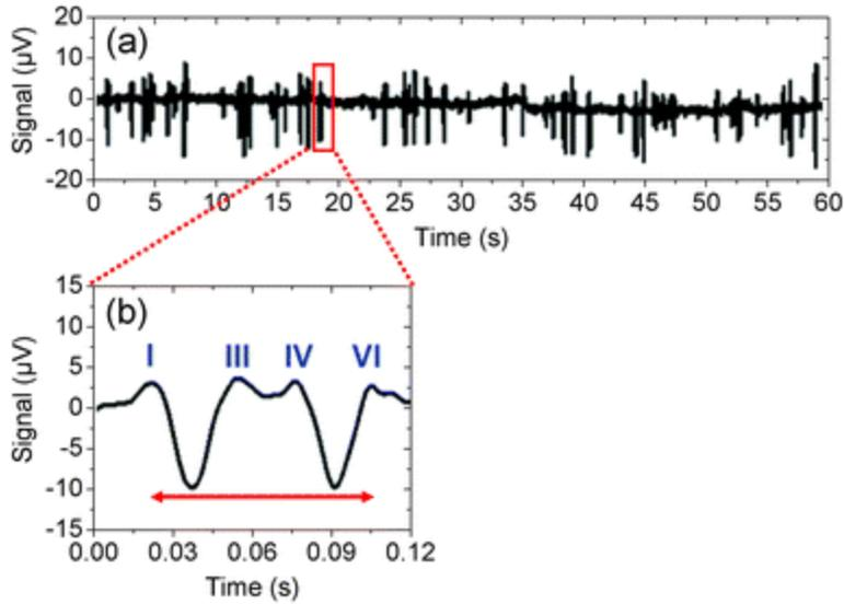
Fig. 2 Signal generated by beads flowing through a coulter counter. a) Pulse train of many beads being detected by the counter b) Zoomed in shot to show pulses caused by two individual beads. Adapted from [17]
