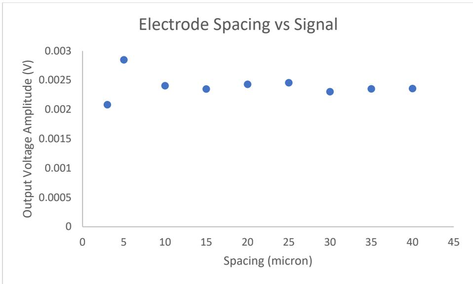
Fig. 14 Spacing between electrodes vs output voltage amplitude for second of the bipolar peaks
