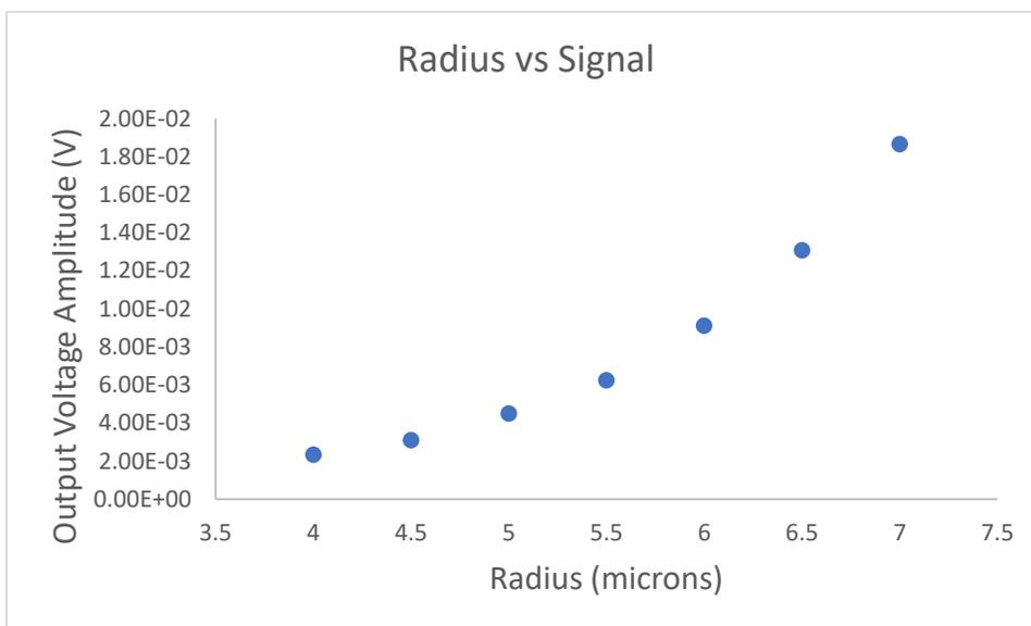
Fig. 11 Particle radius vs output voltage amplitude for second of the bipolar peaks
