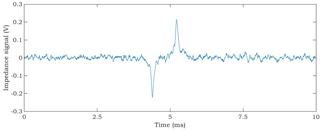
Fig. 20 Signal Produced in experimental tests with 7 micron diameter polystyrene beads
