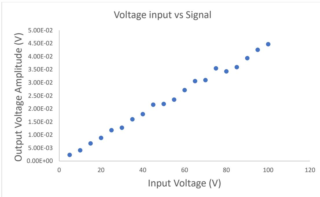
Fig. 10 Input voltage at middle electrode vs output voltage amplitude for second of the bipolar peaks
