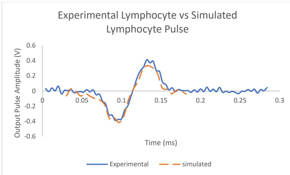
Fig. 18 A comparison of curve shape for experimental lymphocyte results vs simulated lymphocyte results. Simulated results were transformed by multiplying amplitude by 160. Additionally, the x-position parameter in the simulated results was converted to time by the following formula:  $t=(pos-50)/330$  so that it could best match up with the experimental curve
