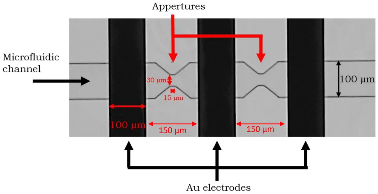
Fig. 5 Another chip design used for comparison simulations. Adapted from [28]
