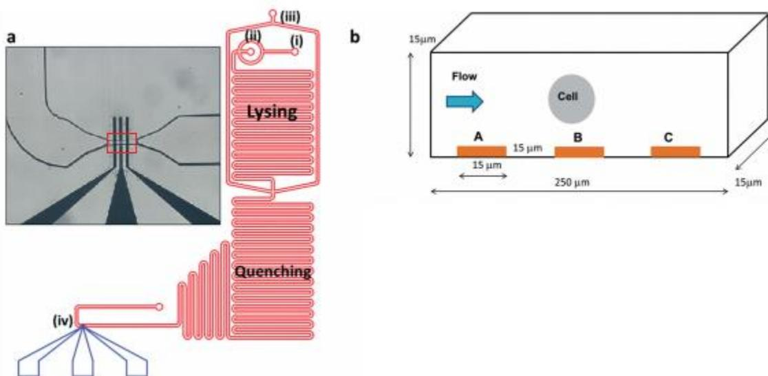
Fig. 4 a) Design of chip used as base for simulations, specific area modeled is outlined in red. b) Diagram of layout of counting channel. A, B, and C are electrodes, with voltage being input through electrode B. Adapted from [27]
