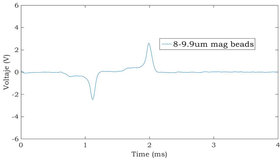
Fig. 21 Signal produced in experimental tests with 8-9.9 micron diameter magnetic beads
