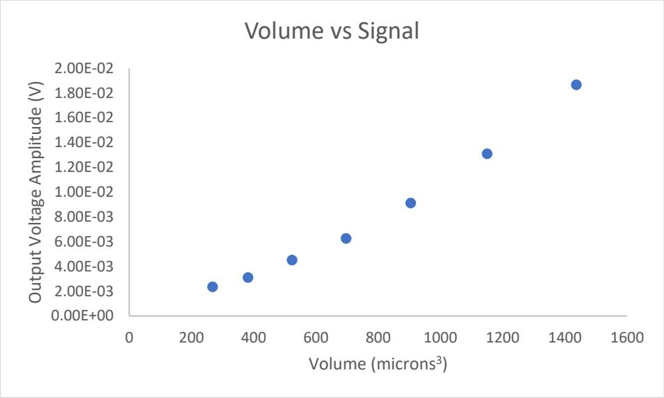
Fig. 12 Particle volume vs output voltage amplitude for second of the bipolar peaks. Volume numbers obtained by converting from radius using volume of a sphere
