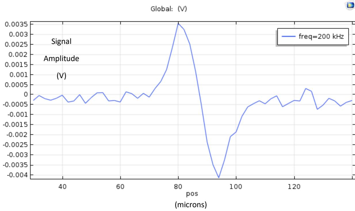
Fig. 17 Graph of voltage difference against x position for Magnetite Shell test. Pulse is inverted compared to tests where outer layer is composed of low conductivity material such as the pulse in Fig. 6
