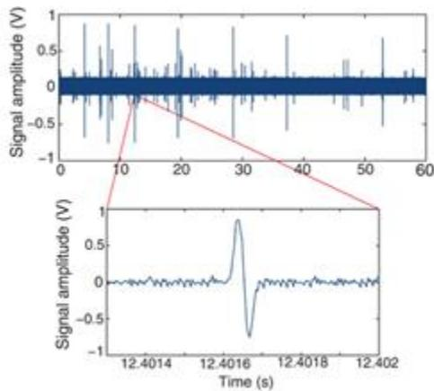
Fig. 3 Typical bipolar pulses obtained by microfluidic coulter counter as cells flow over electrodes. Top image shows multiple pulses in sequence and bottom image isolates an individual example of the bipolar pulse. Adapted from [12].
