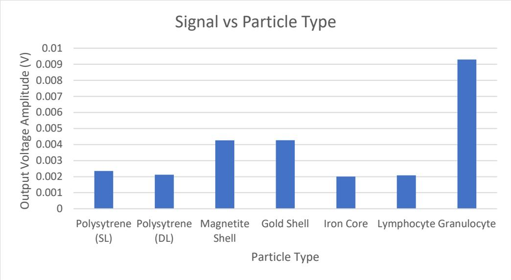
Fig. 16 Particle types vs output voltage amplitude for second of the bipolar peaks. Types were: polystyrene single layer (Polystyrene (SL)), polystyrene double layer (Polystyrene (DL)), polystyrene core with magnetite shell (Magnetite Shell), polystyrene core with gold shell (Gold Shell), iron core with polystyrene shell (Iron Core), Lymphocyte cell (Lymphocyte), and Granulocyte cell (Granulocyte)
