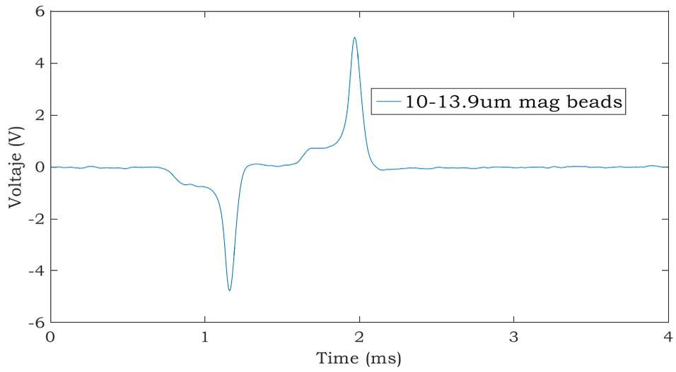
Fig. 22 Signal Produced in experimental tests with 10-13.9 diameter micron magnetic beads
