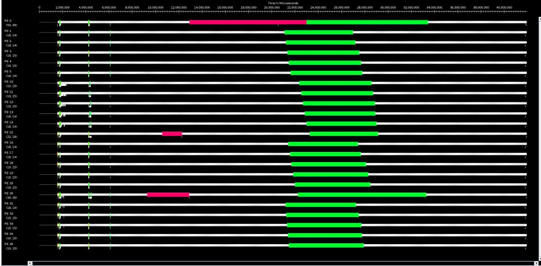
Figure 4.1: Projections timeline view of Phase III with map-based reducers. The horizontal axis shows time in microseconds and the vertical axis represents the timeline for each PE. The red regions indicate the time spent inside reducer functions for merging maps contributed by different PEs. The green regions show the time taken to distribute and rebuild the final merged map on each PE.
