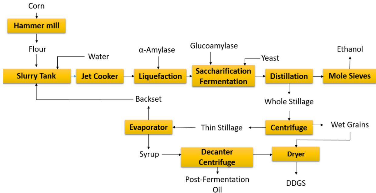
**Fig 2.1. Schematic of dry grind ethanol process.**
