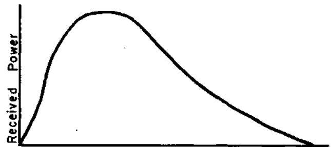
(b.) Received power curve when radar antenna is directed along AB.
