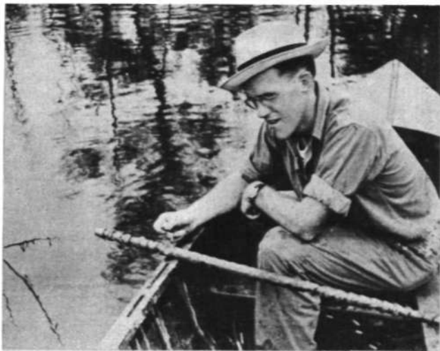
FIG. 4. USE OF SPUD IN MEASURING SEDIMENT THICKNESS.
