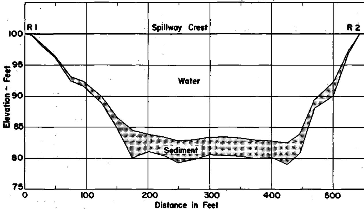
FIG. 5. CROSS SECTION OF RANGE R1-R2.
