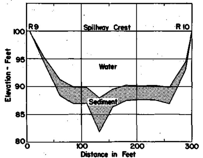
FIG. 6. CROSS SECTION OF RANGE R9-R10.
