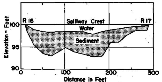
FIG. 7. CROSS SECTION OF RANGE R16-R17.
