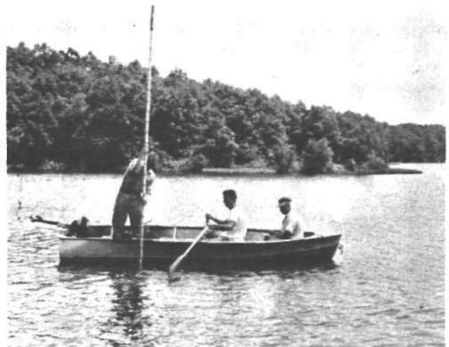
FIG. 3. USE OF THE SOUNDING POLE IN MEASURING SEDIMENT.
