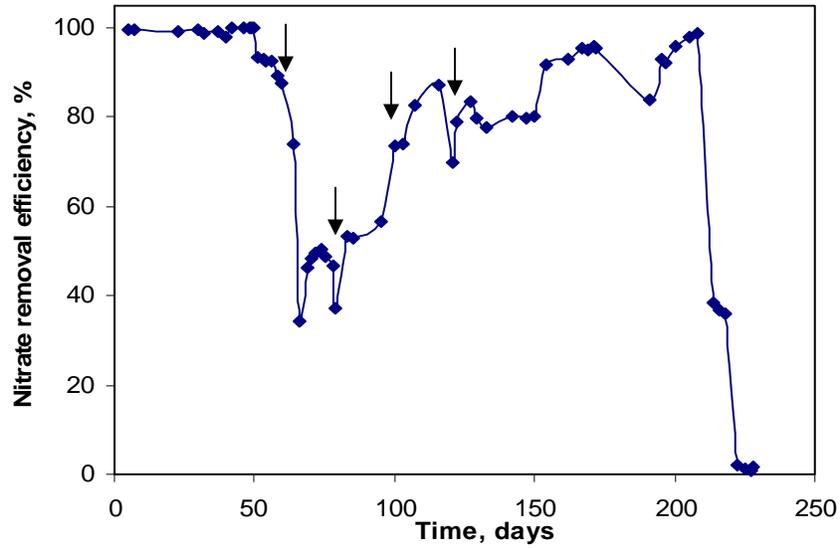
**Figure 2.9** Time course of nitrate removal in SLAD column reactor 1 during the operational period (228 d). Arrows represents re-inoculation. Response surface column runs started at day 150. Day 0 corresponds to a new inoculation at the beginning of the test.
