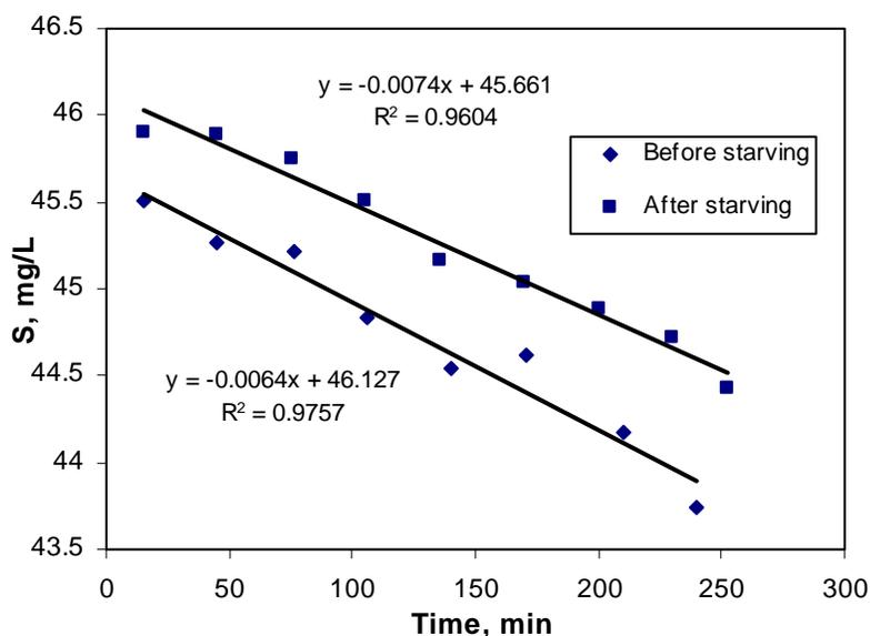
**Figure 3.5** Time course of nitrate-N concentration,  $S$ , in the batch reactor used for  $k_d$  estimation before and after 30-hr starving.
