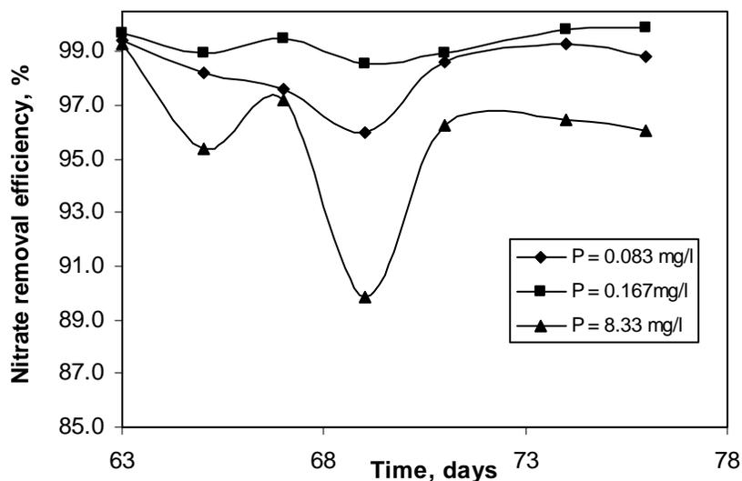
**Figure 2.6 Comparison of nitrate removal efficiency corresponding to different phosphorus concentrations after the feed nitrate-nitrogen concentration increased to 50 mg/l NO<sub>3</sub>-N and the HRT was kept at 6 hours. The feed solution for reactors 1-3 contained 0.083, 0.167 and 8.33 mg P/l, respectively. Day 0 corresponds to a new inoculation.**
