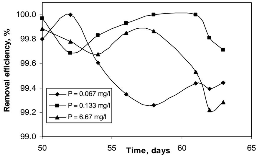
Figure 2.5 Comparison of nitrate removal efficiency corresponding to different phosphorus concentrations after the feed nitrate-nitrogen concentration increased to 40 mg/l  $\text{NO}_3\text{-N}$  and the HRT was kept at 6 hours. The feed solution for reactors 1-3 contained 0.067, 0.133 and 6.67 mg P/l, respectively. Day 0 corresponds to a new inoculation.
