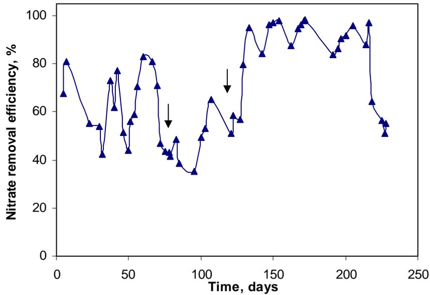
**Figure 2.11** Time course of nitrate removal in SLAD column reactor 3 during the operational period (228 d). Arrows represents re-inoculation. Response surface column runs started at the day 150. Day 0 corresponds to a new inoculation at the beginning of the test.
