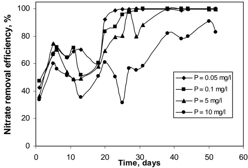
Figure 2.4 Effects of phosphorus concentration in feed solution on nitrate removal efficiency at the influent nitrate-nitrogen concentration of 30 mg/l and the HRT of 6 hours. The feed solution for reactors 1-4 contained 0.05, 0.1, 5, and 10 mg P/l, respectively. Day 0 corresponds to a new inoculation.
