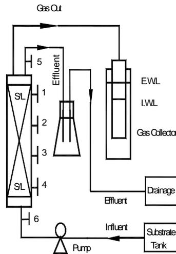
**Figure 2.1 Experimental set-up: upflow fixed-bed SLAD column reactor system. S/L is sulfur/limestone; 1, 2, 3, 4, 5 and 6 are sampling ports; E.W.L.: external water level; I.W.L.: internal water level; there were tap water in effluent flask and acidic salt solution in gas collector.**
