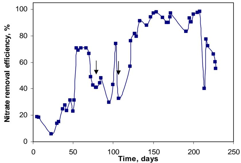
**Figure 2.10** Time course of nitrate removal in SLAD column reactor 2 during the operational period (228 d). Arrows represents re-inoculation. Response surface column runs started at the day 150. Day 0 corresponds to a new inoculation at the beginning of the test.
