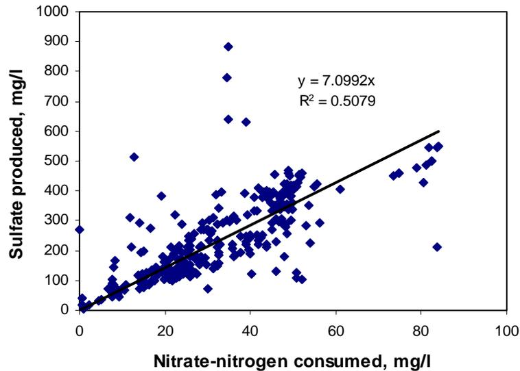
**Figure 2.8 Relationship between sulfate production and nitrate-N reduction in all samples.**
