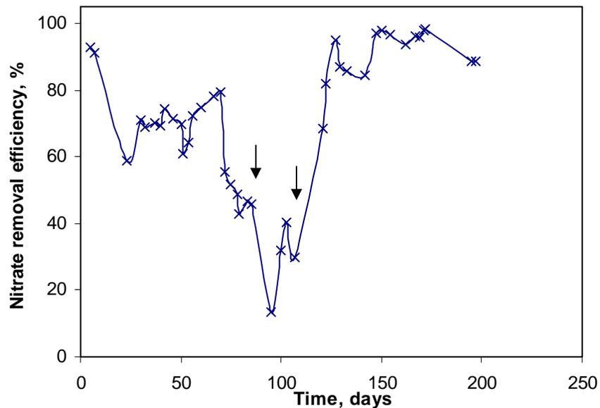
**Figure 2.12** Time course of nitrate removal in SLAD column reactor 4 during the operational period (200 d). Reactor 4 shut down due to system failure by accident at day 198. Arrows represents re-inoculation. Response surface column runs started at day 150. Day 0 corresponds to a new inoculation at the beginning of the test.
