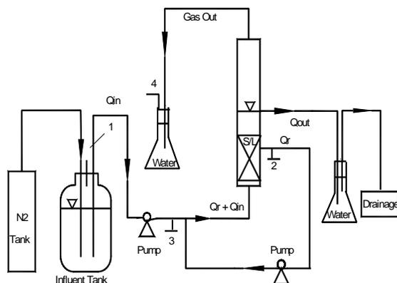
Figure 3.1 Experimental set-up for kinetics study. (Note: 1 and 4 are N<sub>2</sub> gas vents; 2 and 3 are sampling ports.)
