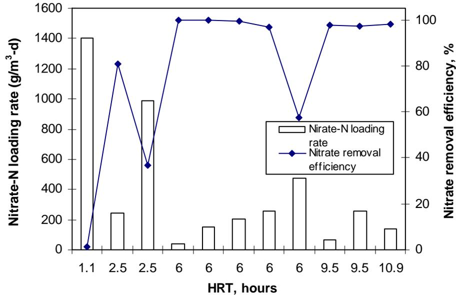
**Figure 2.7 Relationship among nitrate removal efficiency, nitrate loading rate, and HRT.**
