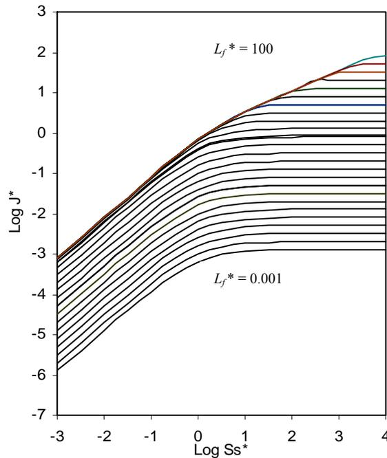
**Figure 3.2 Family of dimensionless curves. (From bottom to top  $L_f^*$  is 0.001, 0.0016, 0.0025, 0.0040, 0.0064; 0.01, 0.016, 0.025, 0.04, 0.064; 0.10, 0.16, 0.25, 0.40, 0.64; 1.0, 1.6, 2.5, 4.0, 6.4; 10, 16, 25, 40, 64, and 100, respectively; the thick black curve  $L_f^* = 1$ .)**
