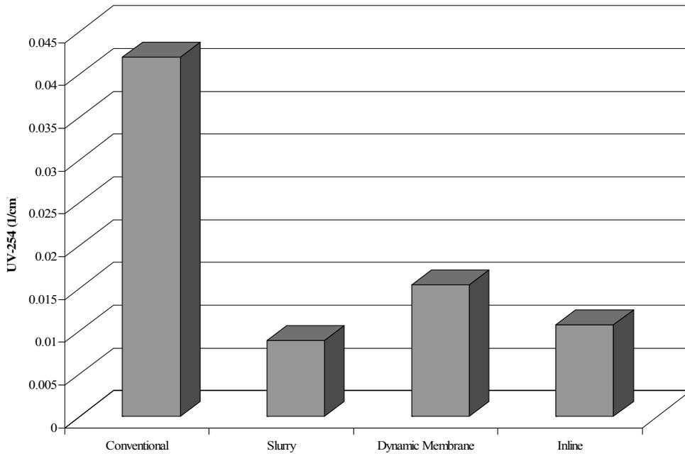
**Figure 16: Comparison of UV-254 values for membrane fouling.**
