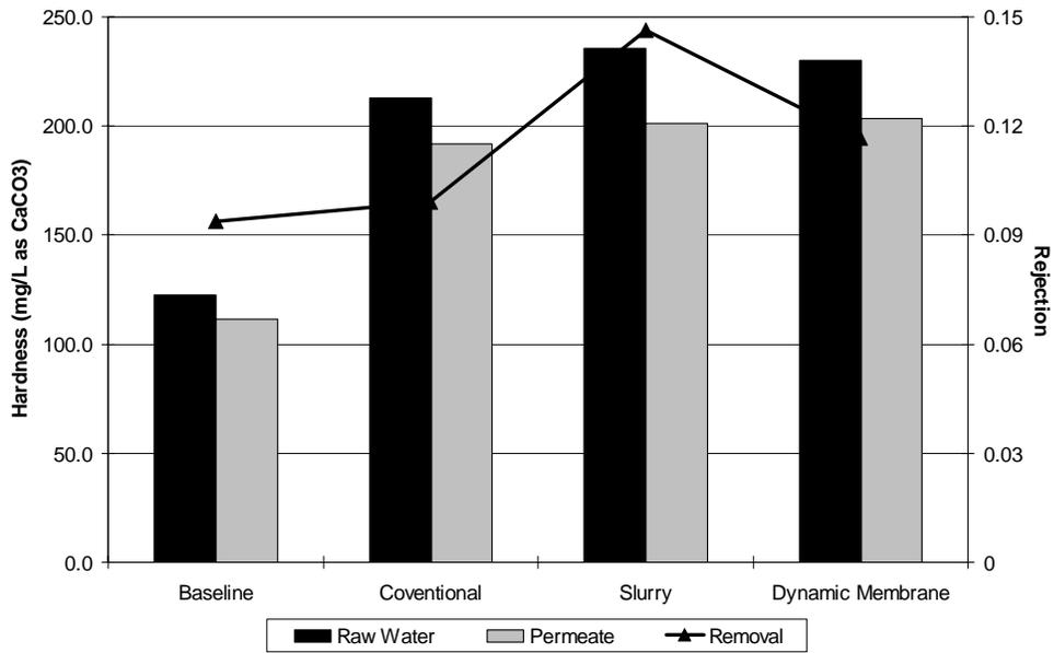
Figure 11: Comparison of hardness values between each test.
