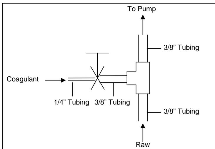
**Figure 2: Inline Setup**
