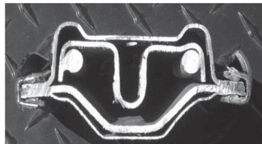
Figure 1. "B" posts showing rods.
