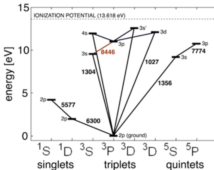
Figure 1: Partial Grotian diagram of atomic oxygen, where the 8446 Å transition highlighted.
