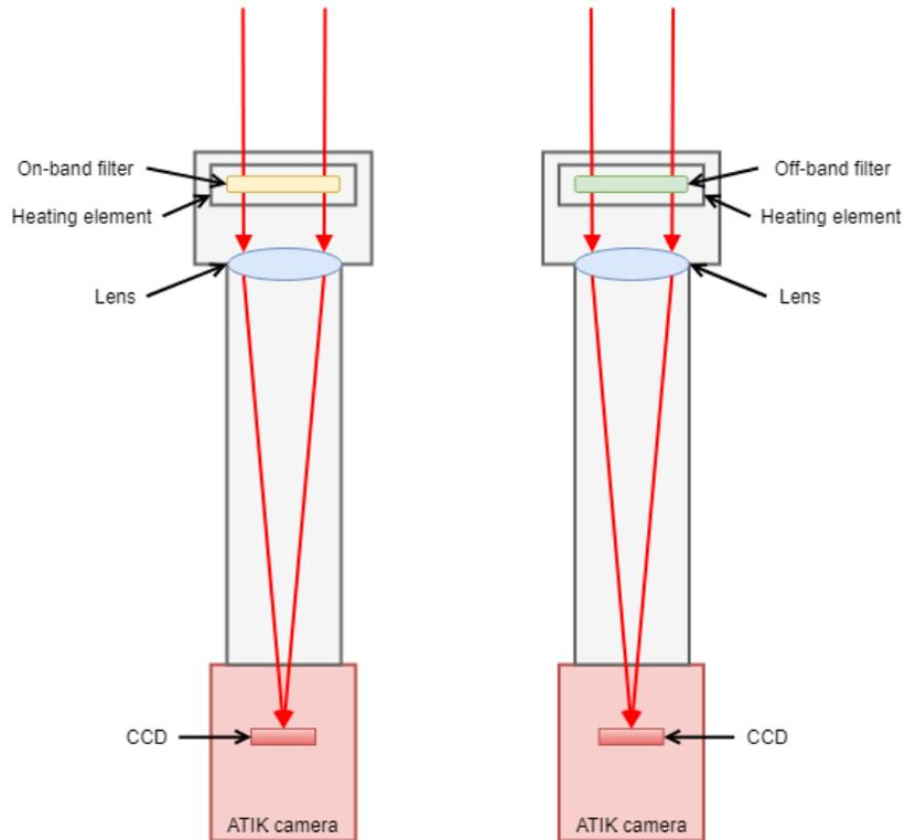
Figure 4: Optical path of the photometers.
