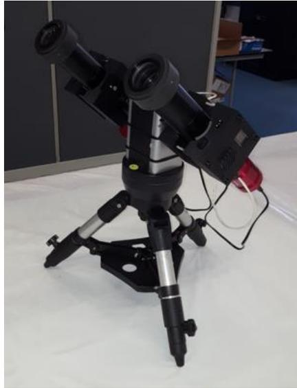
Figure 3: The two-channel photometer.
