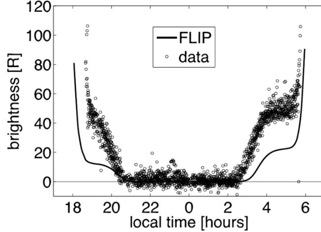
Figure 2: 844.6nm emission data and FLIP PE model calculations, winter at Arecibo Observatory, 1999 – 2002 [2].
