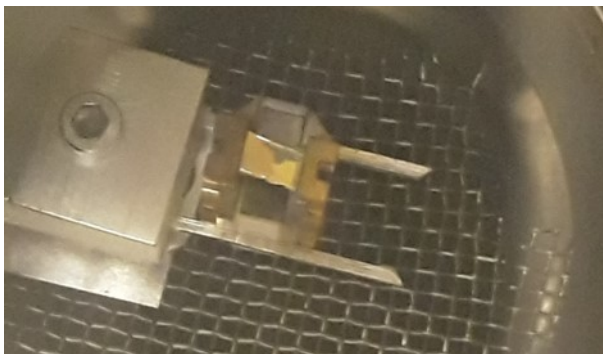
Figure 2.2: STM Sample-holder with Au(111) Surface and Si Backing
