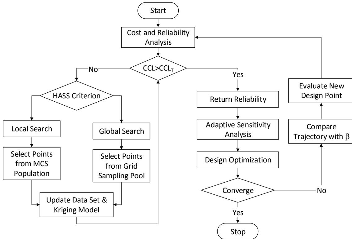
**Figure 5.** Flowchart of developed HASS methodology and the ASA method for RBDO
