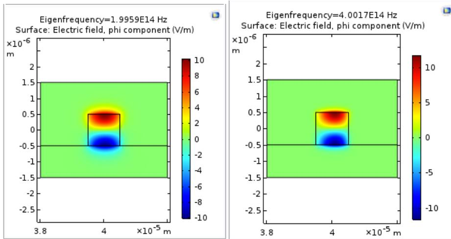
Figure 2.1: TM Mode Azimuthal Electric Field inside Ring Cross Section
