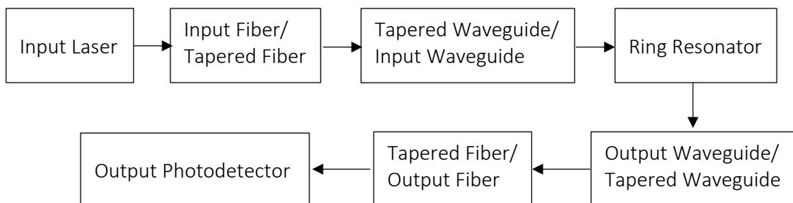
Figure 1.1: Wavelength Conversion Block Diagram
