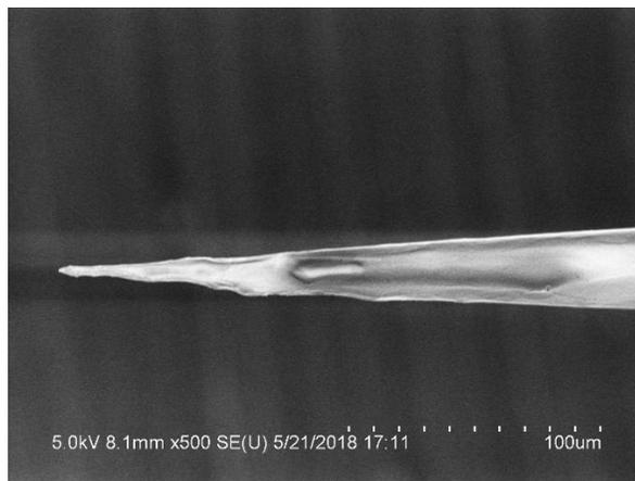
Figure 4.1: The Taper Fiber Tip Image
