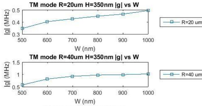
Figure 2.2:  $|g|$  vs.  $W$  of 350 nm Thick Rings with 20  $\mu\text{m}$  and 40  $\mu\text{m}$  Radius
