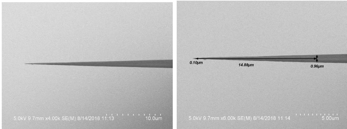
Figure 4.2: The Tapered Tip Image Formed in an Acid with O-xylene
