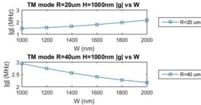
Figure 2.3:  $|g|$  vs.  $W$  of 1  $\mu\text{m}$  Thick Rings with 20  $\mu\text{m}$  and 40  $\mu\text{m}$  Radius
