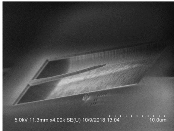
Figure 3.3: The Released Tapered Waveguide
