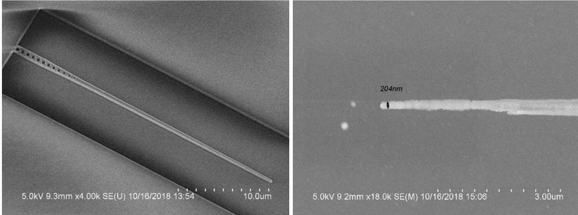
Figure 3.2: The Tapered Aluminum Nitride SEM Image
