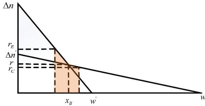
**Figure 2.** Detailed illustration of base carrier profile. The shaded area represents the QW region.
