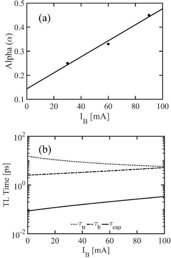
**Figure 5.** (a) Dependence of current transport factor  $\alpha$  on the base current  $I_B$  in the HBTL with one QW ( $m=1$ ) in the base of Ref [3]. The experimental data are represented as the dots. (b) Capture time  $\tau_{cap}$  (solid curve), transit time  $\tau_{tr}$  (dotted curve) and base lifetime  $\tau_b$  (dashed curve) as a function of base current  $I_B$  for HBTL.
