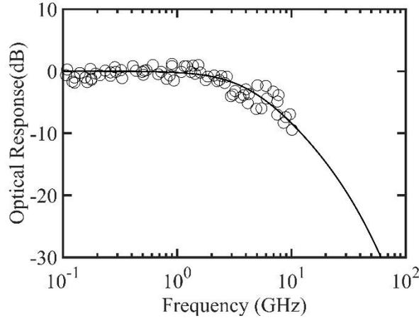
**Figure 4.** Small signal frequency response of the LET. The -3 dB frequency falls at ~4 GHz. The experimental data [22] are represented in dots.
