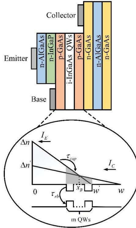
**Figure 1.** Schematic of the layered HBLET structure (upper diagram) with the minority carrier profile (lower diagram) in the transistor base caused by the QW capture. The emitter and the collector are on the left and right side of the base, respectively. The shaded area in the lower diagram indicates the minority carrier concentration above the m-QWs.  $w$  and  $x_B$  denote the base width and the middle point of QW location, respectively.
