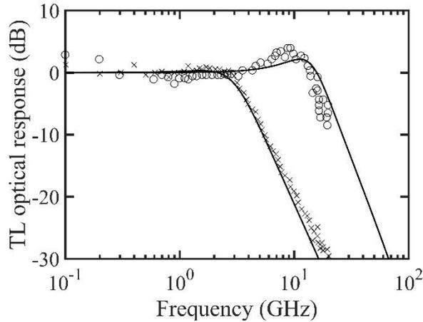
**Figure 6.** Small signal frequency response for HBTL. The -3 dB frequency falls at ~4 GHz. The left curve represents the frequency response at  $I_b = 30 \text{ mA}$ ,  $\alpha = 0.25$  and the curve on the right represents frequency response at  $I_b = 90 \text{ mA}$ ,  $\alpha = 0.45$ . The experimental data are represented in dots and crosses.
