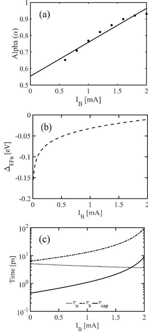
**Figure 3.** (a) Dependence of current transport factor  $\alpha$  on the base current  $I_B$  in the HBLET consisting of 2 QWs ( $m=2$ ) in the base of Ref [22]. The experimental data are represented as the dots. (b) Quasi-Fermi level with respect to the ground level  $\Delta E_{Fn}$  as a function of  $I_B$ . (c) Capture time  $\tau_{cap}$  (solid curve), transit time  $\tau_{tr}$  (dotted curve) and base lifetime  $\tau_b$  (dashed curve) as a function of base current  $I_B$  for HBLET.
