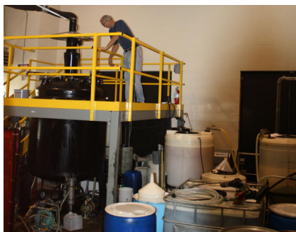
Joe Pickowitz working with the biodiesel pilot plant that was set up at ISTC's testing facilities.
