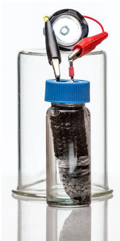
An LED light is lit by the corn cob biochar supercapacitor. (Photo by L. Brian Stauffer - U. of I., (University of Illinois) News Bureau)
