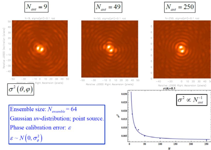
Figure 1. Statistical imaging simulation of interferometric phase errors.
