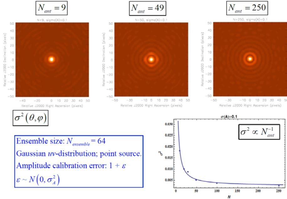
Figure 2. Statistical imaging simulation of amplitude errors.
