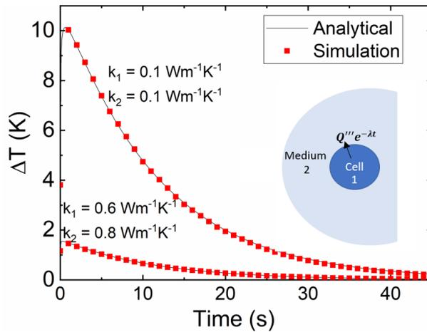
Figure S1. Validating the finite element model for a generalized transient heat. The transient temperature change ( $\Delta T$ ) at the center of the cell is plotted. The temperature changes for two different combinations of cell ( $k_1$ ) and medium ( $k_2$ ) thermal conductivity are shown. The inset schematically depicts the domain of analysis, which is a cell of radius  $a$ , dissipating heat in an infinite medium.
