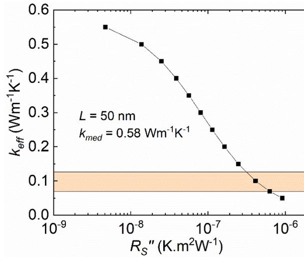
Figure S2. A high resistance  $R_s''$  reduces the effective thermal conductivity  $k_{eff}$ . The  $R_s''$  shown here corresponds to a length-scale  $L=50$  nm and  $k_{med}=0.58$  Wm<sup>-1</sup>K<sup>-1</sup>. The shaded region corresponds to a  $k_{eff}$ : 0.07 – 0.13 Wm<sup>-1</sup>K<sup>-1</sup>, which was recently reported [4] to be the range of effective thermal conductivity at intracellular regions.
