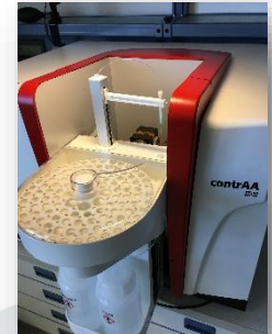
contrAA 800 HR-CS-GFMAF system (Analytik Jena AG, Jena, Germany)
