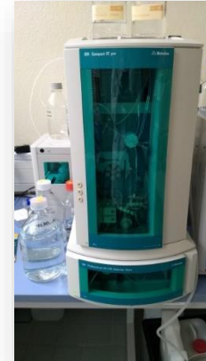
881 compact IC pro system (Metrohm GmbH & Co. KG, Filderstadt, Germany)
