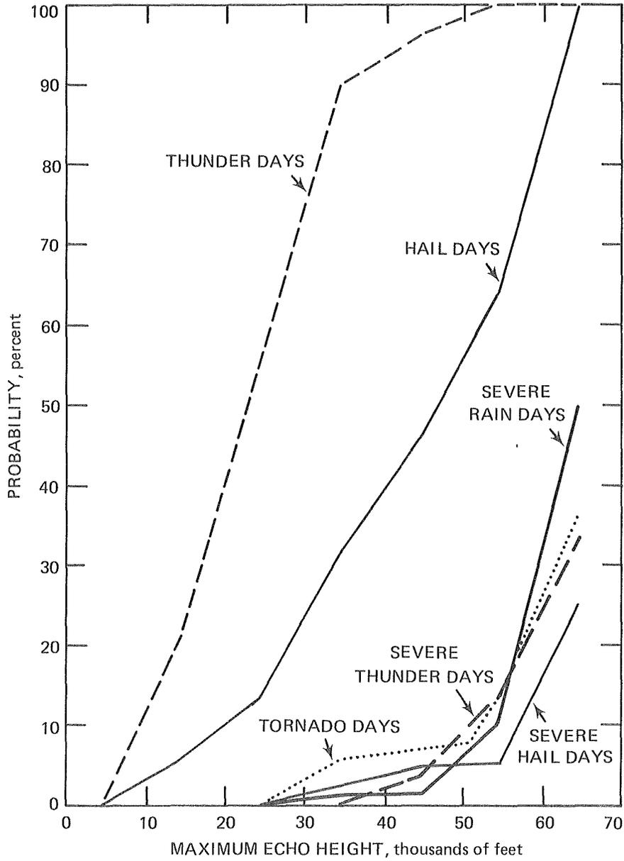
Daily severe weather probabilities as a function of maximum radar echo top heights.
