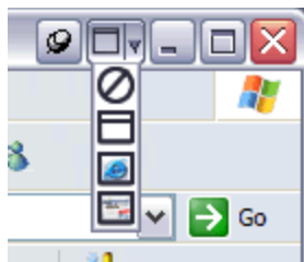
Figure 5. Two additional buttons appear on the title bar of each application. The leftmost button allows users to "pin" an application so that it cannot be relocated by other users. The adjacent button allows the user to specify how the application can be represented in other users' interfaces. The options are invisible , outline only , icon , or thumbnail views.
