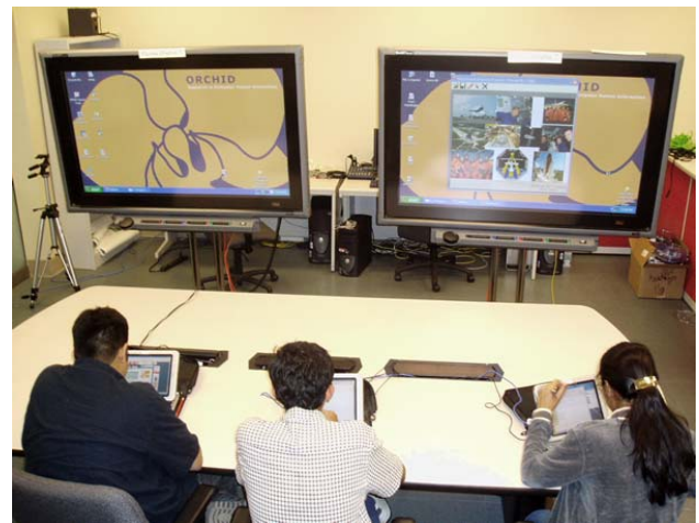
Figure 1. A group of users performing the collage activity in our MDE. Each user is individually searching for images using several open Internet Explorer windows on a tablet PC. When a desirable image is found, the user relocates the shared canvas (shown on the right-most large display) to the local tablet to add the image. The user may then relocate the canvas back to a large display or directly to another user's tablet.
