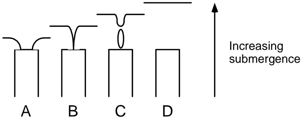
Figure 9 – Vortex Dependence on Submergence [11]
