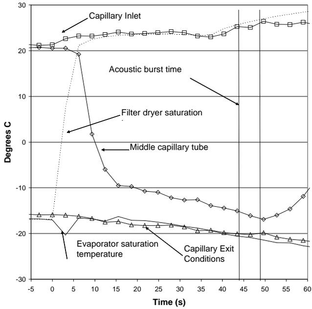
Figure 4 – No Warming of Suction Line Heat Exchanger (Acoustic Burst)
