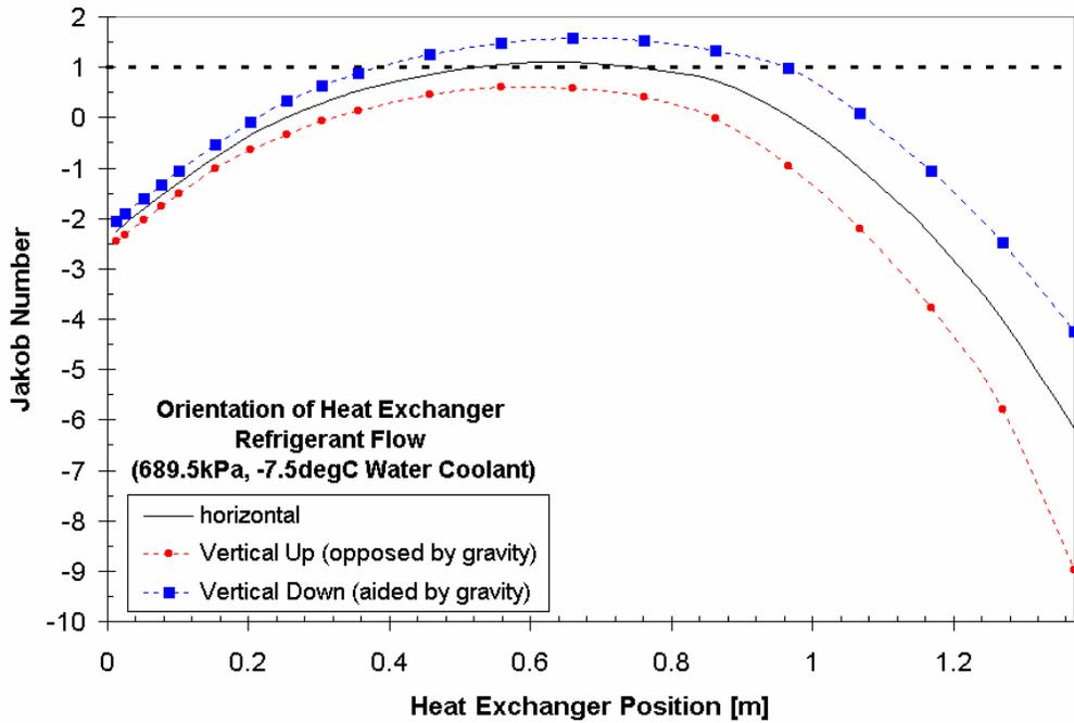
Figure 12 – Effect of Heat Exchanger Orientation
