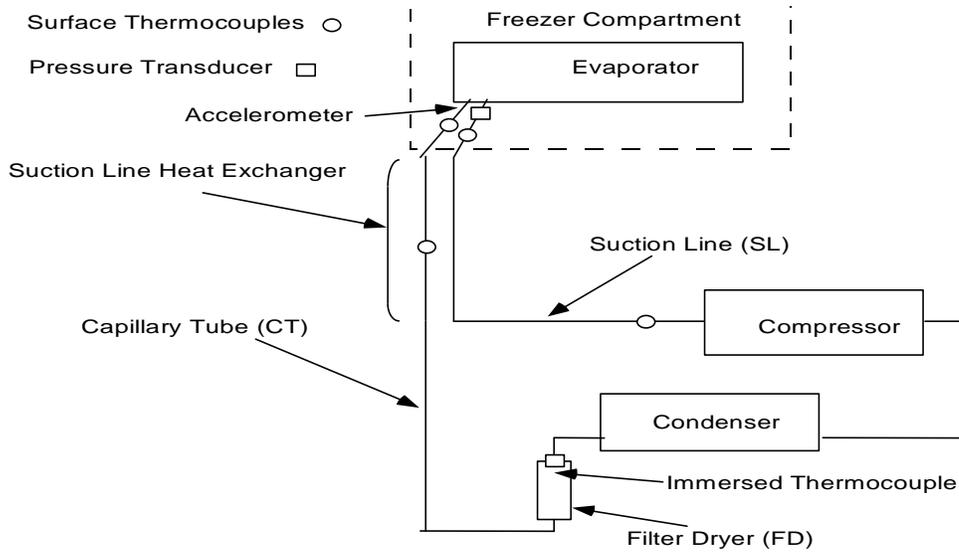
Figure 13 – Household Refrigeration Line Test Schematic
