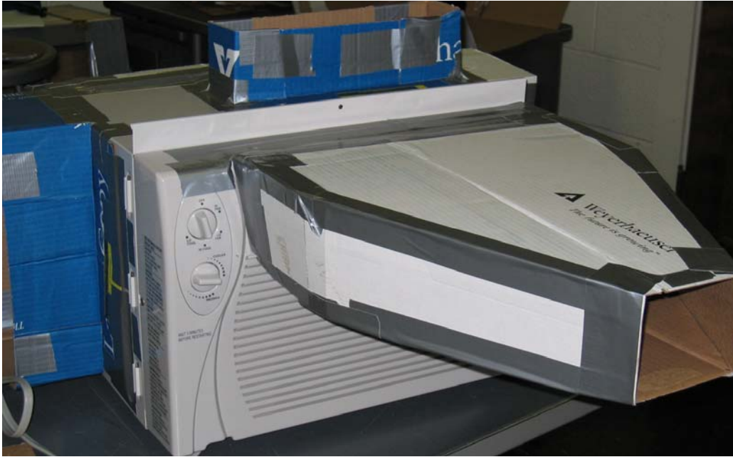
Figure 2.4 Unit while energy balance was performed.
