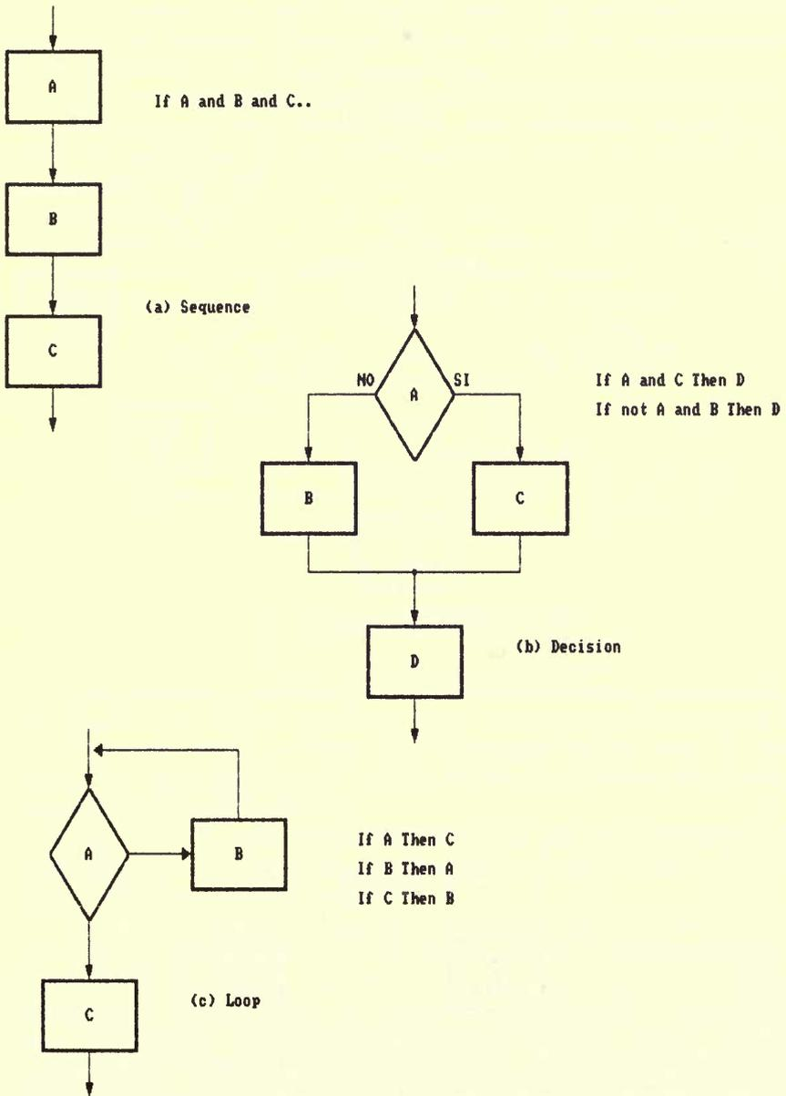
Figure 1. Conversion to production rules of the three basic building blocks of structured flowcharts
