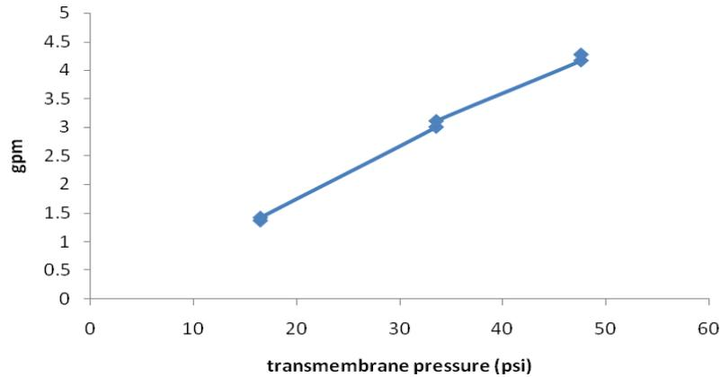
**Figure 4: Warm Conditioned Water Flux.**
