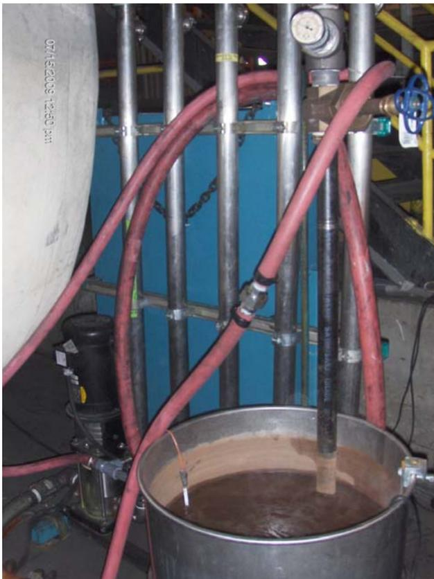
**Figure 5: UF Pilot.** The stainless steel barrel (foreground) is the process/concentration tank. Condensate enters the process tank by means of a gravity-fed inlet pipe (not shown) from the autoclaves. Then it is pumped throughout the membranes (five vertical metallic pipes) and leave as either permeate (foreground red tubing) or as retentate (black vertical pipe into the process tank) where it is further concentrated and reprocessed through the system.
