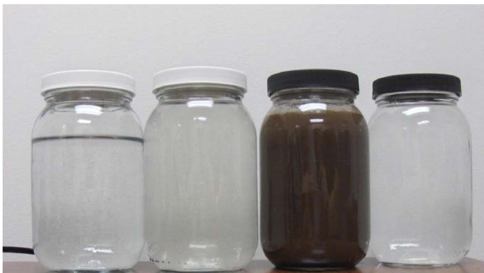
**Figure 7: (Left to Right) Samples of conditioned water, initial feed, end retentate, and end permeate.**
