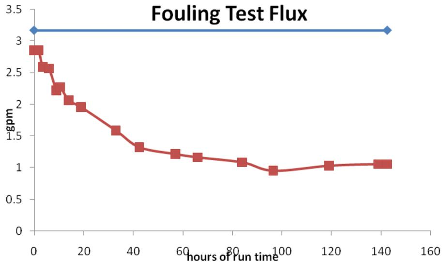
**Figure 6: Fouling Test Flux-** the blue line is the conditioned water flux (control) and the red line is the condensate permeate flux rate over time.
