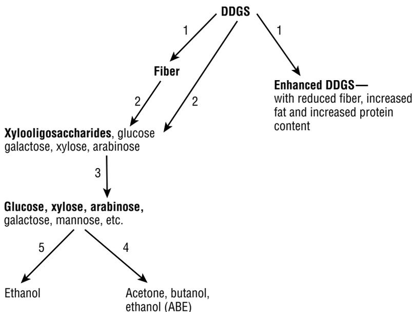
**Figure 1** Pretreatment and conversion of DDGS to value-added products. 1 = elusieve process (Srinivasan et al. 2005); 2 = electrolyzed water pretreatment (Wang, Feng, and Luo 2004); 3 = enzymatic hydrolysis; 4 = ABE fermentation by solventogenic clostridia (Ezeji, Qureshi, and Blaschek 2004); 5 = ethanol fermentation by *E. coli* FBR 5.
