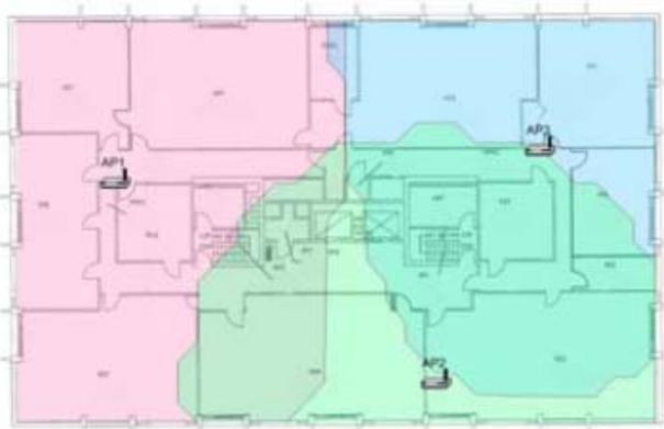
Figure 3. Signal on 4<sup>th</sup> floor from 4<sup>th</sup> floor
