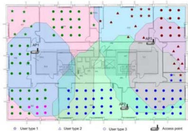
Figure 5. Overall signal coverage and demand node Assignment on the 4<sup>th</sup> floor
