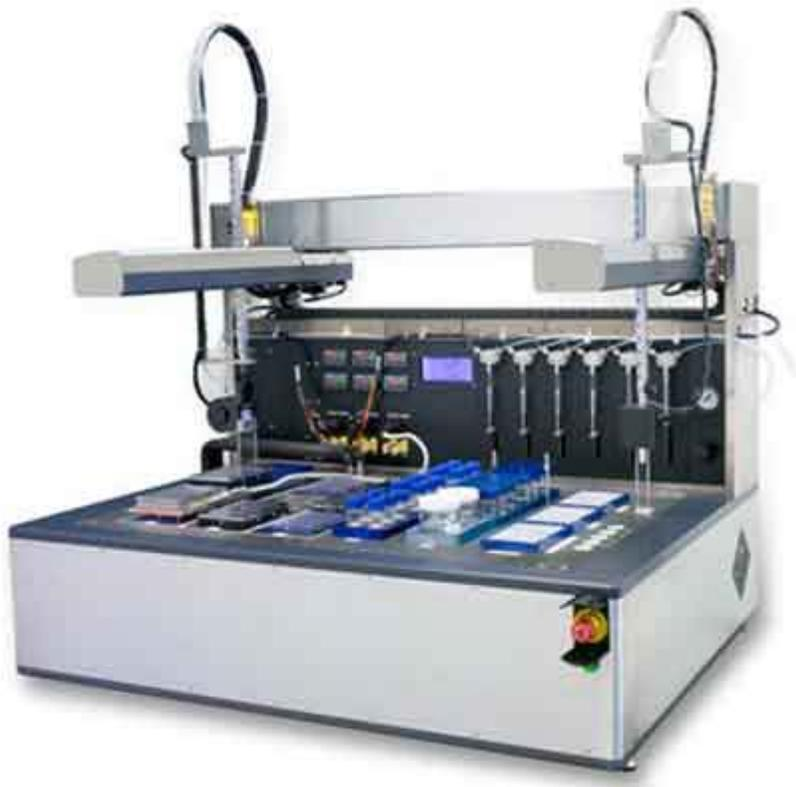
**Figure 1.4** Example of a SYMYX system used for crystallization screening. This highly complex robotic system used robotic pipettes to meter fluids into wells and perform crystallization studies [17].
