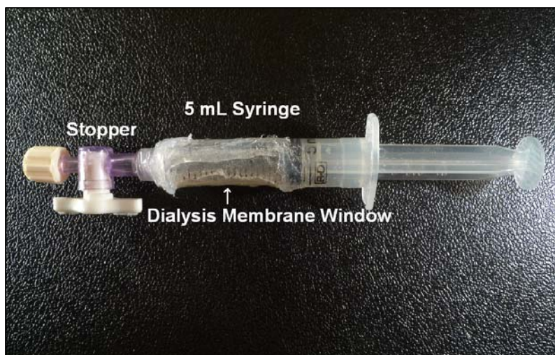
Figure 3: Aqueous chemical sampler ready for deployment.
