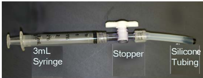
Figure 2: Dissolved Gas Sampler (As described by Vroblesky et al. 2007).
