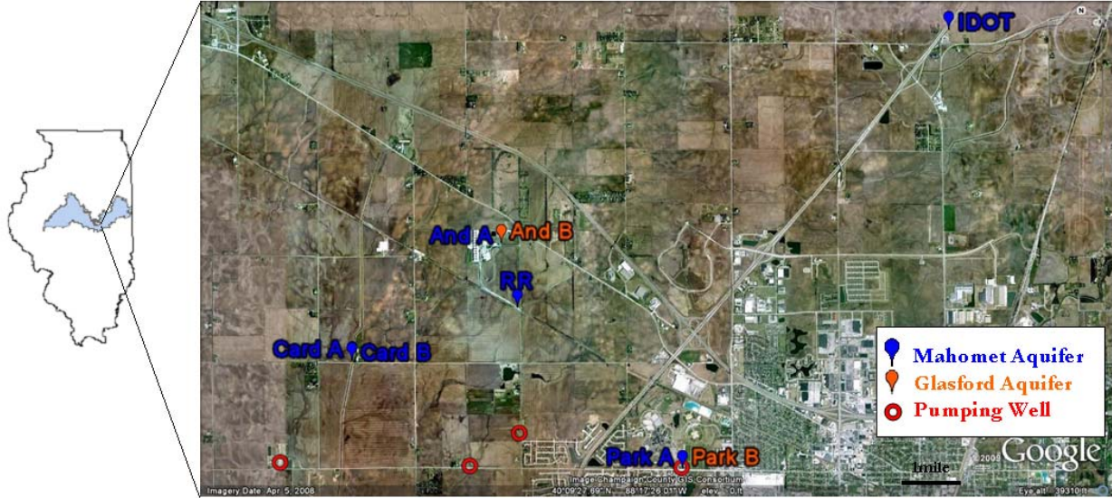
Figure 1: A map of the Mahomet Aquifer indicating locations of monitoring (orange and blue balloons) and production wells (open red circles).
