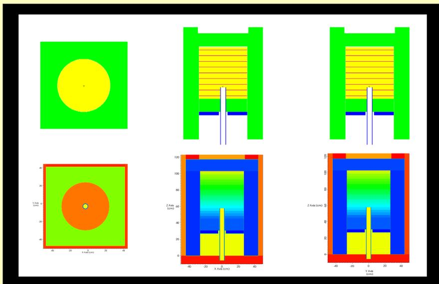
Fig. 1: From left to right, XY-plane, XZ-plane, and YZ-plane slices of geometry from the zeus2 criticality problem using MCNP5 with its plotter (top) and Mercury with VisIt (bottom)
