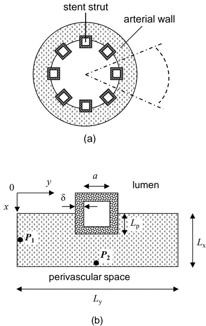
**Figure 1.** (a) Cross-sectional view of a stented vessel. Dashed lines show a reduced domain by symmetry. (b) Extracted rectangular vascular domain with partial embedment of a single stent strut.
