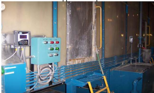
*Photo of Analyzer on left, electrical panel in middle and sensor on far right in tank 4, solenoid not shown.*
