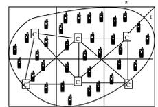
Fig. 1. The mobility area with  $n$  mobile nodes and  $m$  servers (controllers  $C$ )
