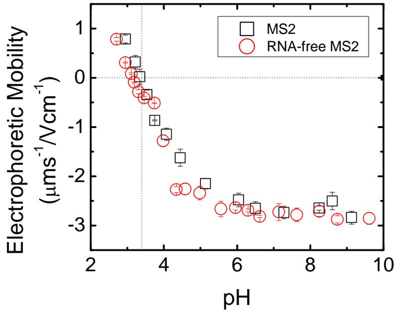
Figure 4: Electrophoretic mobility of wild-type MS2 and hollow MS2 at a constant 1 mM NaCl solution while varying the pH with HCl and NaOH. The isoelectric point was found not to vary significantly between the two types of MS2, as the wild-type MS2 and hollow MS2 was found to be 3.4 and 3.2 respectively.
