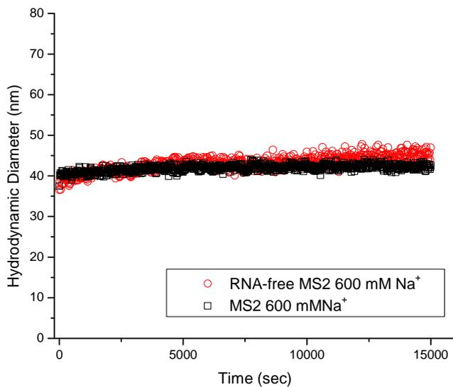
Figure 5: Time resolved dynamic light scattering of MS2 and RNA-free MS2 experiencing aggregation at 600 mM NaCl. Although the aggregation kinetic rates are similar in magnitude, the Kapp of RNA-free MS2 was slightly higher, Kapp of 0.0003 compared to untreated MS2 Kapp 0.0001, suggesting that MS2 behaves as a softer particle.
