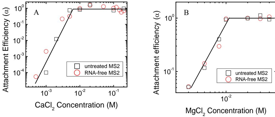
Figure 6: Aggregation bacteriophage particles of MS2 and hollow MS2 were similar in the presence of  $\text{Ca}^{2+}$  (a) and  $\text{Mg}^{2+}$  (b), measured by time resolved dynamic light scattering. The critical coagulation concentration (CCC) occurs approximately 10 mM for both types of particles in the presence of  $\text{Ca}^{2+}$  and  $\text{Mg}^{2+}$ , after which rapid aggregation occurs.
