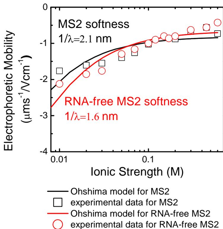
Figure 3: Electrophoretic mobility of MS2 and RNA-free MS2 as a function of ionic strength, using NaCl, at constant pH. This was used to calculate the electrophoretic softness of the MS2 and RNA-free MS2, which were found to be 2.1 nm and 1.6 nm respectively using the Ohshima model (Ohshima 1995). This indicates that the RNA-free MS2 particles were found to be slightly harder particles than the untreated MS2.
