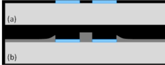
Figure 2.4: A cross section  $\text{SiO}_2$  growth inhibition mask on a GaAs substrate before (a) and after (b) after selective growth of InGaAs layer.
