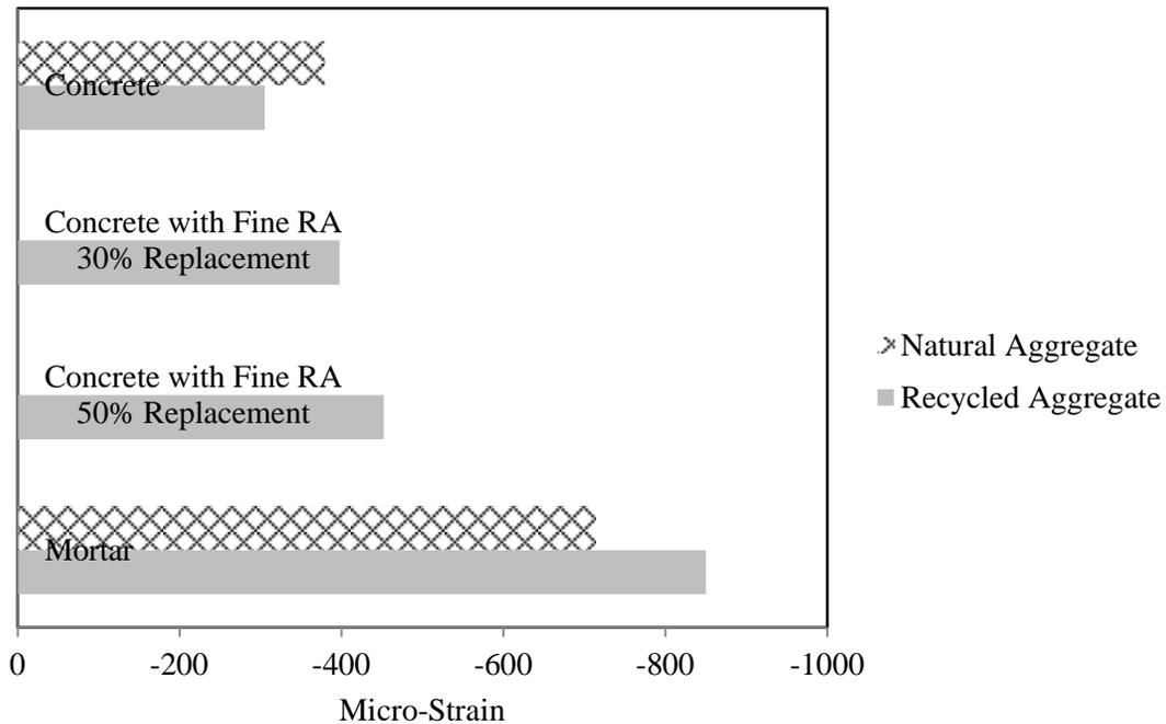
Figure 15. Shrinkage of specimens at 56 days
