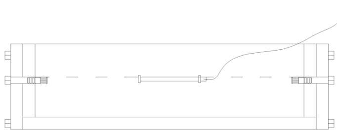
Figure 3. Plane view of mounted embedded gage
