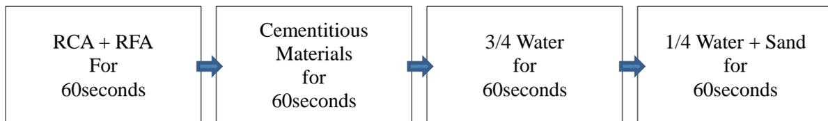
Figure 2. Two Stage Mixing Approach in the experiment
