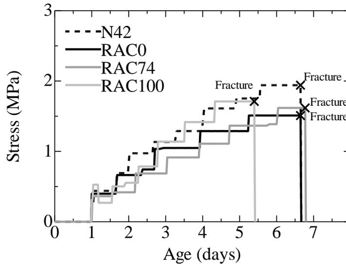
Figure 10. Tensile stress developing of dog bone specimens
