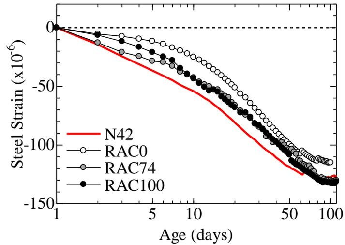
Figure 9. Drying shrinkage of ring specimens
