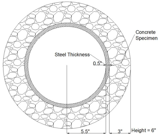
Figure 4. Dimension of ring apparatus
