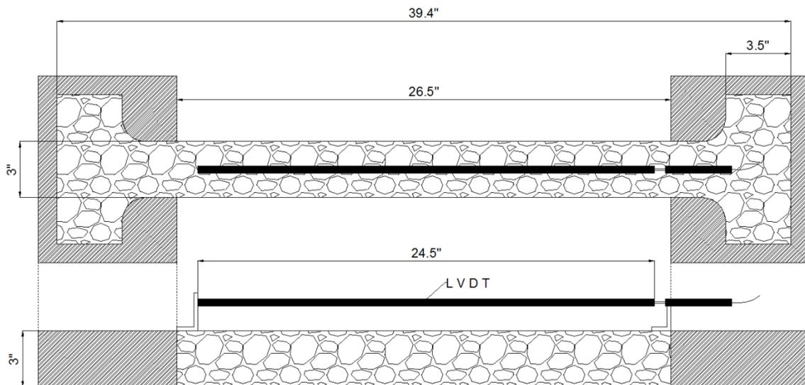
Figure 6. Dimension of dog bone apparatus
