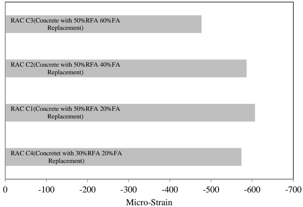
Figure 13. Free shrinkage of series of RAC C at 91days
