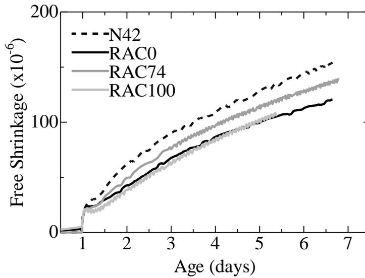
Figure 11. Free shrinkage of dog bone specimens
