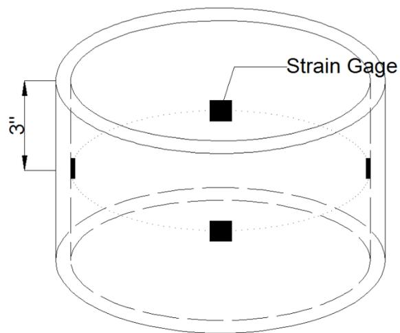
Figure 5. The locations of strain gages
