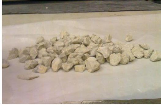
Figure 1. Recycled coarse aggregates
