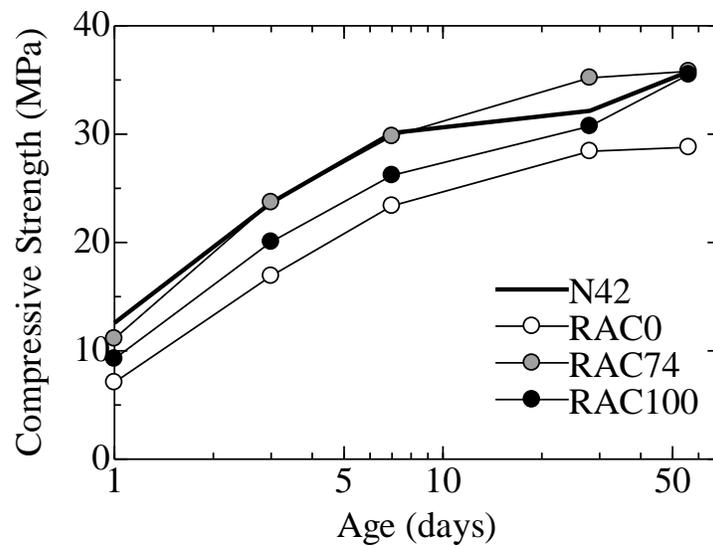
Figure 7. Results of compressive strength of specimens
