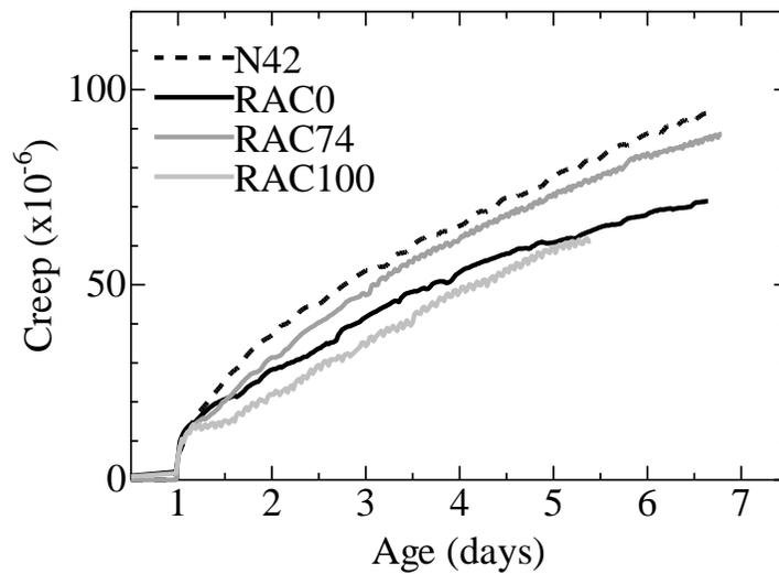
Figure 12. Total creep strain of dog bone specimens
