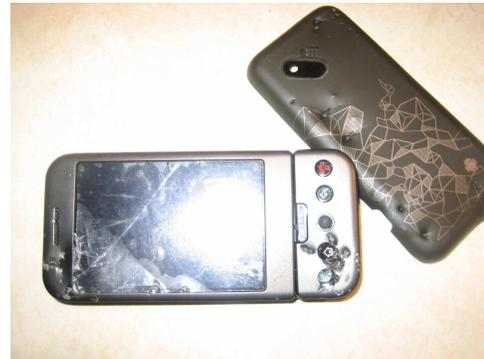
**Figure 1:** Notice the damage to both the screen and the plastic casing.
