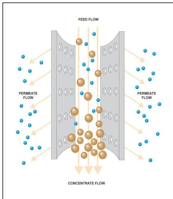
Figure 1: Membrane cross-section
