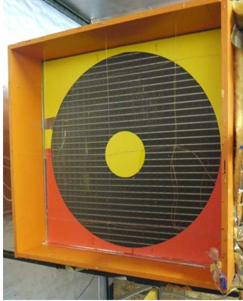
Figure 2.9: The evaporator with poster board used to create a poorly positioned axial fan. The “corners” are with the four corner pieces. The “center” condition is with the yellow circle in the center in addition to the four corners.
