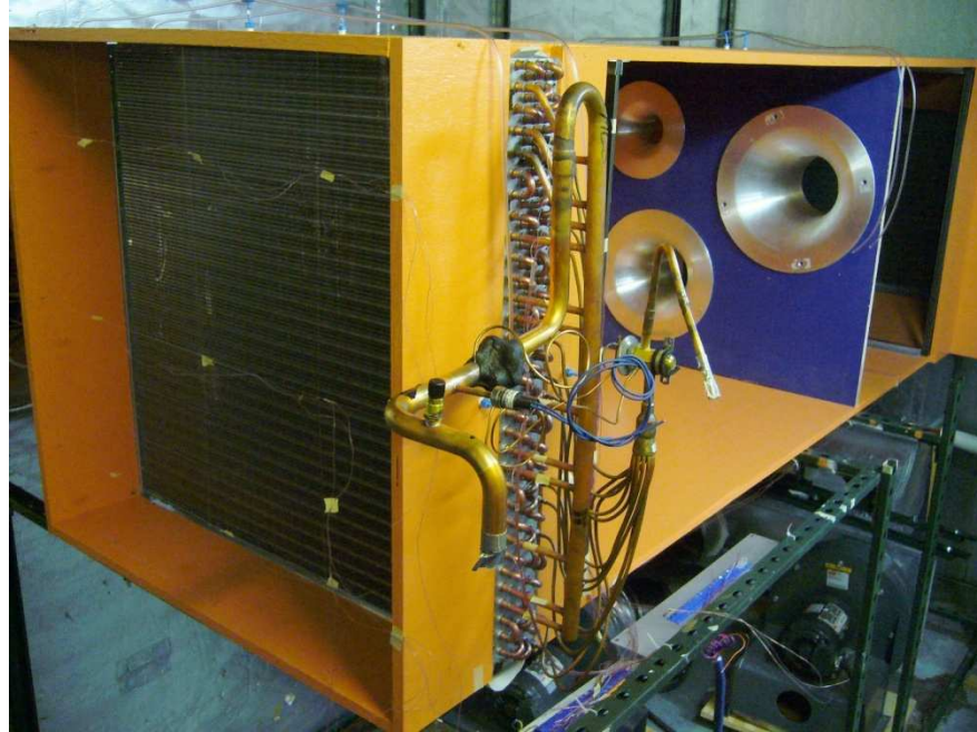
Figure 1.5: Overview of the evaporator, TXV, and distributor in the wind tunnel which has been opened showing the airflow nozzles downstream
