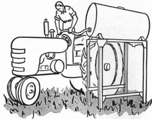
vary as little as possible. This will keep moisture condensation at a minimum. The fuel outlet should be a few inches above the bottom. After filling the storage tank, let the fuel settle before refueling the tractor. Pump fuel directly from storage to the tractor tanks — never use open containers.
