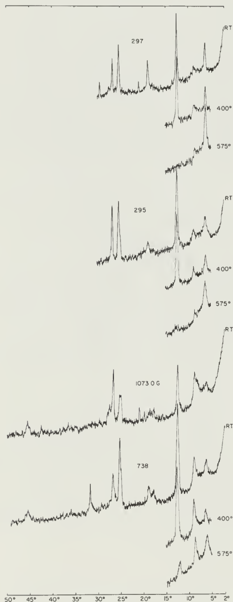
Fig. 4 - X-ray diffraction patterns of chlorite.
