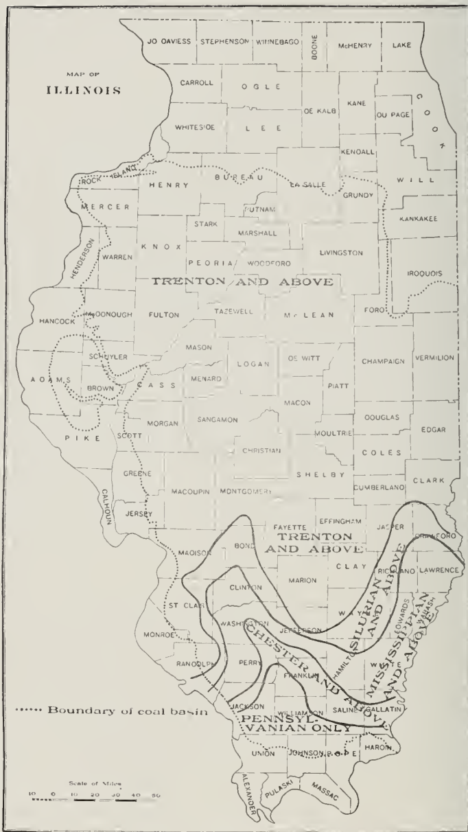
FIG. 5. Horizons with oil possibilities according to carbon ratios.
