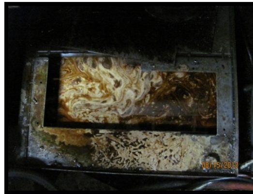
Photo 4: Machine sump of metalworking fluid with tramp oil and other contaminants used in the pilot
