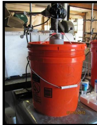
Photo 2: 5-gallon container with housing, membrane, motor, and stirrer
