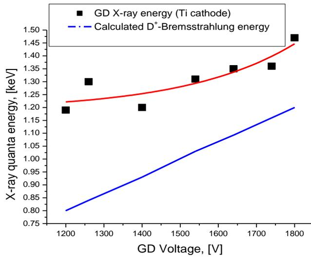
Figure 23: Mean x-ray energy versus glow discharge voltage. Points are the measured energy. The blue curve is the x-ray energy estimated, in assumption of ion induced Bremsstrahlung.
