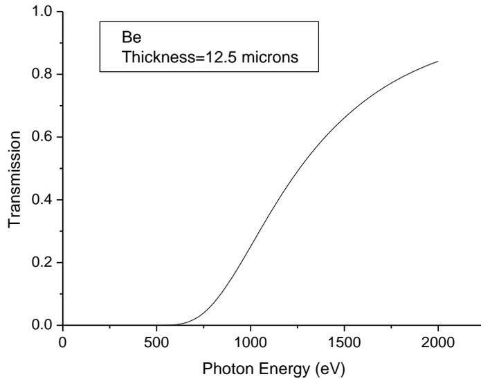
**Figure 15: Filter transmission rate as a function of photon energy.**
