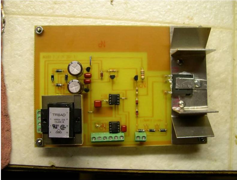
Figure 2: The 2.2-kVA power supply is shown. The circuit board controlling the frequency operates between 100 Hz and 1800 Hz and the pulse width modulation operates with duty cycles from 5% to 95%.
