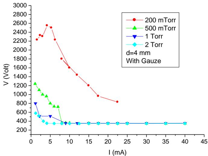
Figure 7: Steady-state applied voltage Paschen curves for configuration 3.
