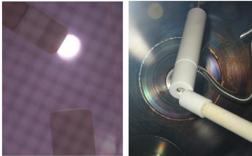
Figure 4: The Basic configuration is shown (left). A photo of the discharge is presented (right). The large volume UIUC chamber allows space for internal diagnostics.
