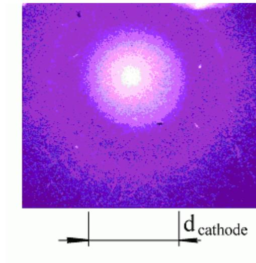
Figure 20: Image of x-ray emission from the cathode using the pinhole camera. The objective is narrowed by use of a  $15\mu\text{m}$  Be shield in front of the camera, showing a bright center spot. Conditions of discharge –  $J = 150\text{mA}$ ,  $U = 1250\text{ V}$ ,  $p = 5.3\text{ mm Hg}$ , the exposure time –  $1000\text{ s}$ . The spot diameter is equal to the cathode size [3].
