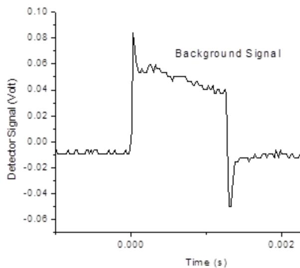
Figure 18: Background signal with detector blocked with copper foil. A background level of  $\sim 0.06$  V occurs at the start of the pulse and slowly falls to  $\sim 0.04$  V.
