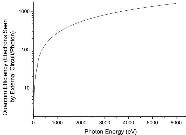
Figure 14: Quantum efficiency of the AXUV 100.
