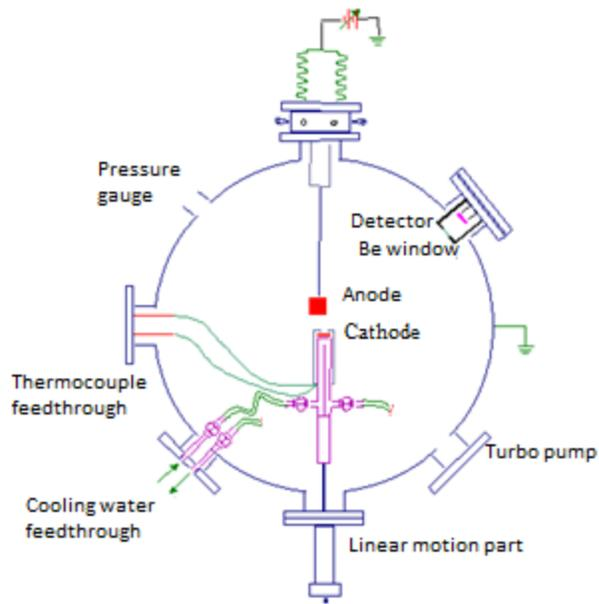
Figure 3: The large volume UIUC chamber gives room for internal diagnostics and thus the anode/cathode separation is easily adjusted.
