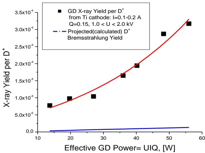
Figure 22: X-ray yield per deuteron in glow discharge versus effective discharge power: points are the experimental yield. The blue curve is the x-ray yield calculated, in assumption of ion induced Bremsstrahlung.
