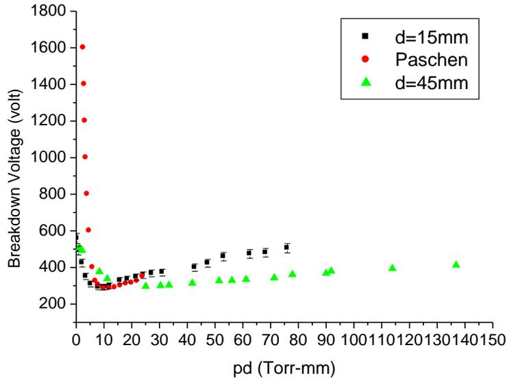
Figure 5: Ideal Paschen curve and the pd-V curve for basic configuration.
