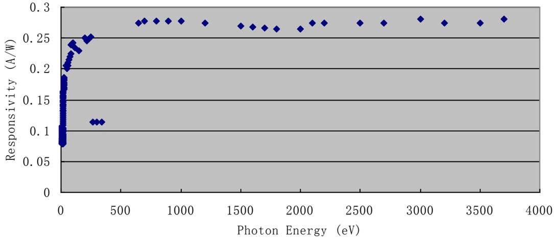
Figure 13: Responsivity of the AXUV photodiodes to photons 100.
