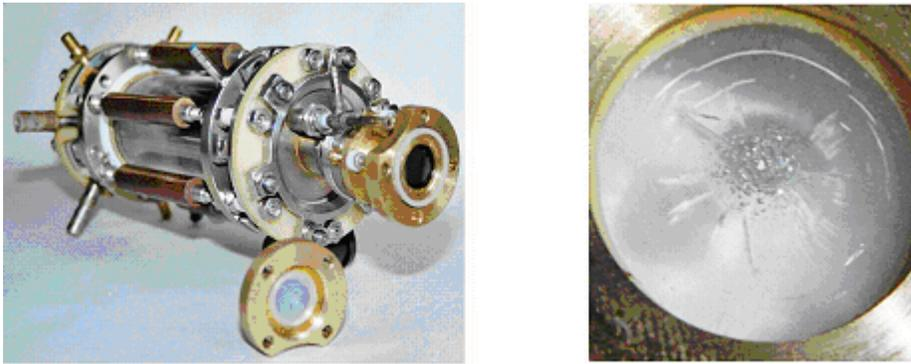
**Figure 1: Photo of Karabut’s prototype X-ray laser device (left) and photo detailing the accumulated damage to plastic target from laser operation (right). The damage pattern appears to be caused by many small beamlets rather than a solid beam.**
