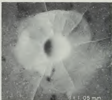
Fig. 4 - Photograph of an indentation in reflected light showing characteristic fracture pattern of fine-grained limestones. Light is shining from left to right and "d" is the diameter of the indentation.
