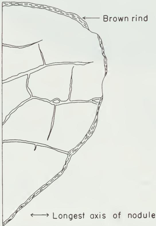
Fig. 3 - Horizontal section of part of sideritic nodule showing laddering of syneresis cracks. Actual size.
