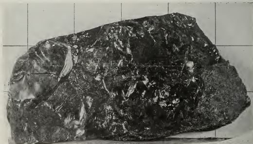
FIG. 5 LUMP OF ILLINOIS COAL THAT WAS BROKEN THROUGH A VITRAIN BAND
