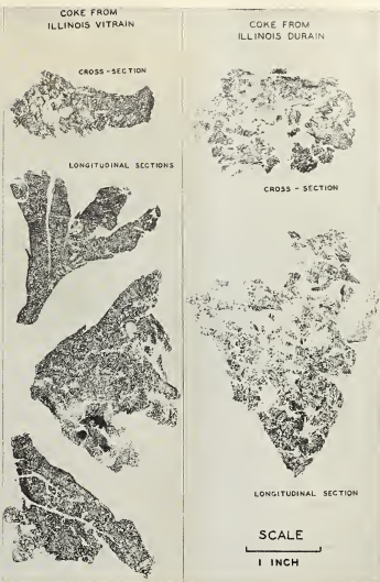
FIG. 3 SECTIONS OF COKE EMBEDDED IN PLASTER OF PARIS TO SHOW DIFFERENCES IN STRUCTURE
