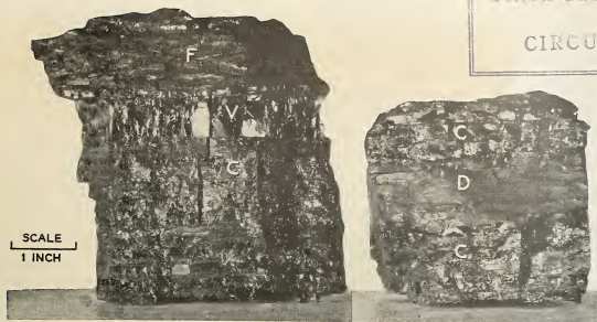
FIG. 1 TWO BLOCKS OF BANDED COAL FROM SOUTHERN ILLINOIS (The four components, clarain, durain, fusain, and vitrain, are indicated by the letters C, D, F, and V, respectively.)
