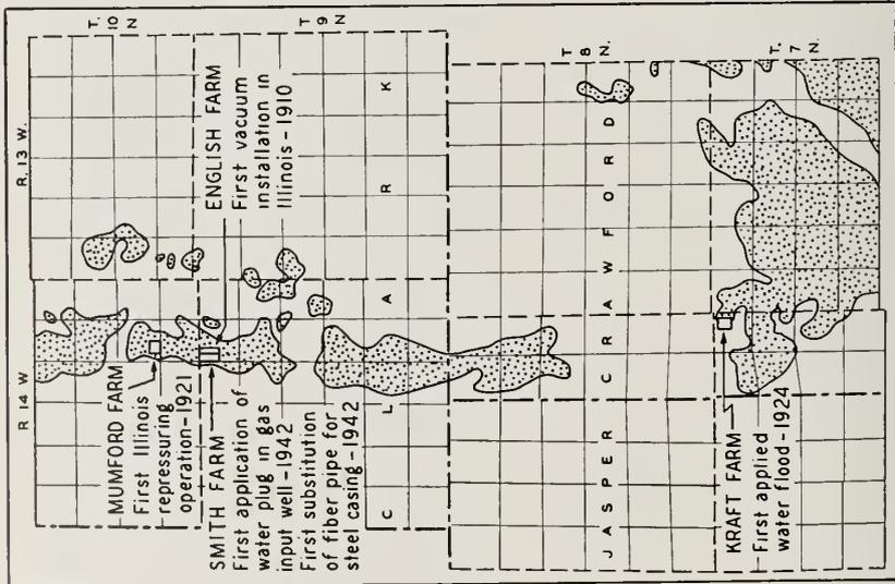
Fig. 1: Map showing location of resaturating experiment. It also shows the initial applications in the state of repressuring, flooding, and nonferrous well casing, these being the work of the author
