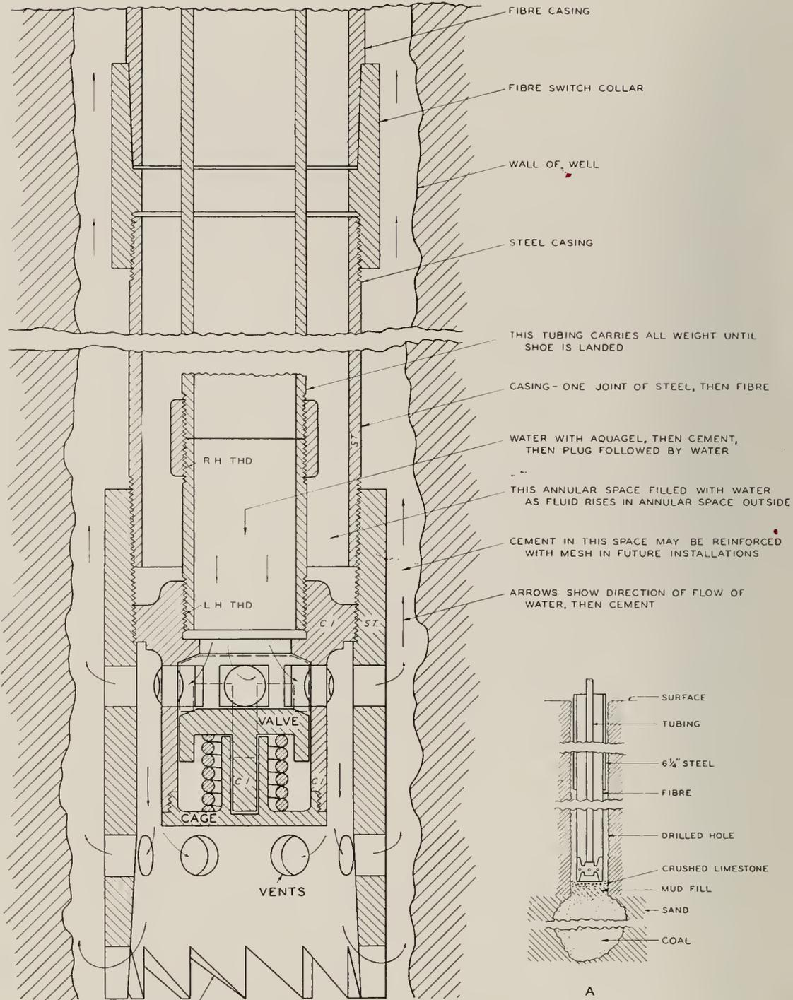
SERRATED TO HOLD WHEN TUBING IS REMOVED BY TURNING OUT OF LEFT HAND THREAD
