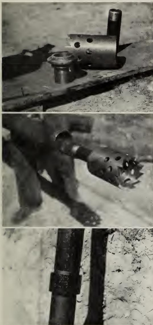
ABOVE: Shoe and adapter run on bottom of fibre pipe. MIDDLE: Shoe made up on tubing ready to be slipped over bottom of fibre pipe. BELOW: A joint of the fibre pipe coupled with a fibre switch collar to a joint of steel pipe.
